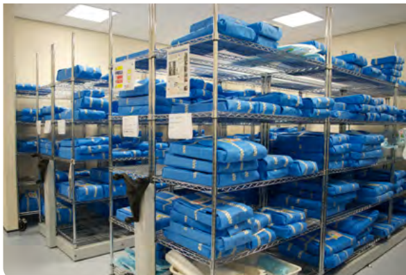
Wire shelving was mounted onto mobile shelving chassis to help create a high density Sterile Store.
