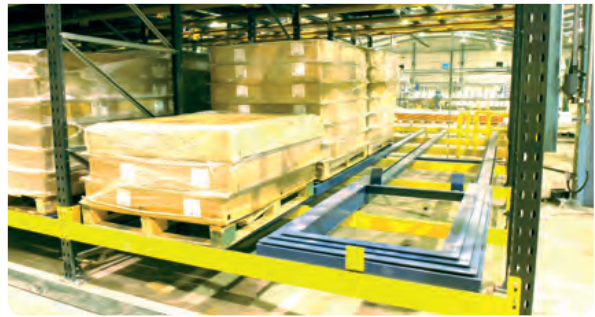
Pallets are loaded onto wheeled carts or rollers and are pushed back along inclined beds. When a load is retrieved the remaining pallets roll forward into position at the picking face
