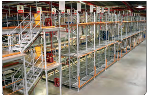
Pick towers can have live storage and garment hanging integrated within the structure, making it a favourite of fashion retail distributors.
